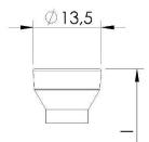
Cylindrical head with Countersinking
