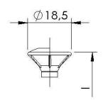
Flat countersunk head 90° with and without raised head, with and without milling ribs
