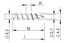
With and without thread variation, with milling ribs
