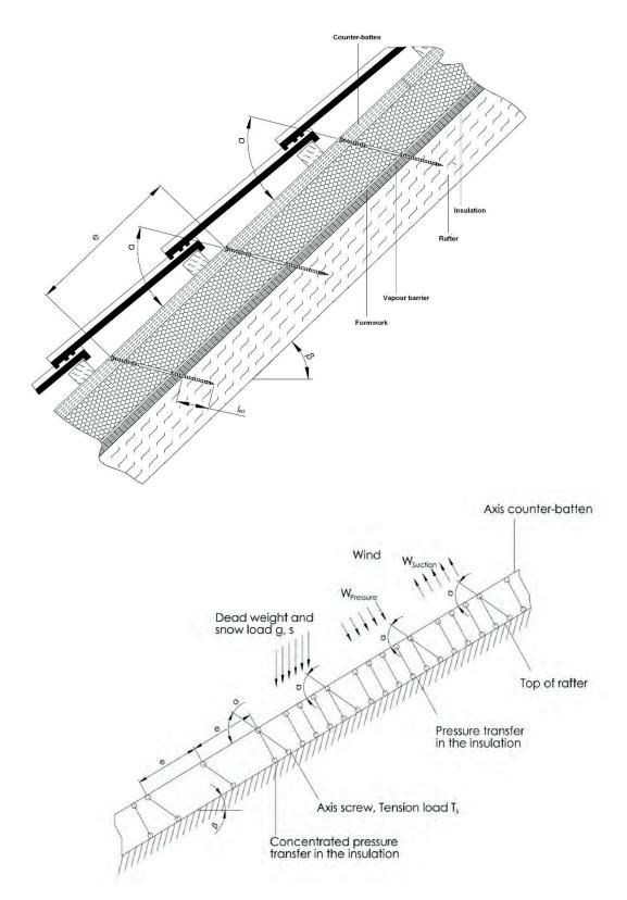
Figure 7: Fastening of the thermal insulation material on top of rafters - structural system for parallel inclined screws
