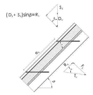
Figure 9: Point loads F<sub>s</sub> perpendicular to the battens, load application in the area of the screw heads
