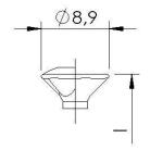
Flat countersunk head 90° with and without raised head, with and without milling pockets
