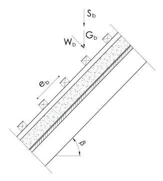
Figure 8: Point loads  $F_b$  perpendicular to the battens
