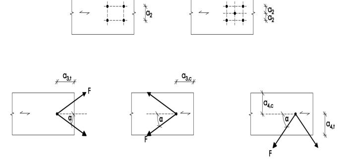
Figure 1: Definition of spacing, end and edge distances in the plane surface
