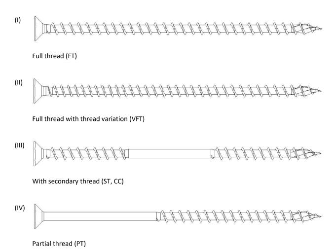
The length and the thread of the screw can be increased optionally up to the maximum thread or screws length, for fixations of insulation or insulation boards, covered with various materials like metal, timber or wood-based panels, fastened at a distance to the timber substructure or in case of fastening in dowels. The respective lengths are shown in the following annexes.
